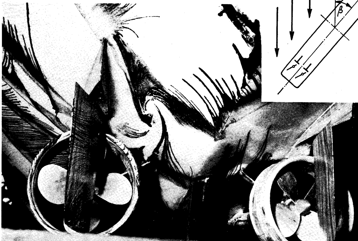
Result of streamline test carried out under oblique flow, \beta = 40 deg, \delta_R = 20 deg (phase when checking the helm), HSVA 1977
