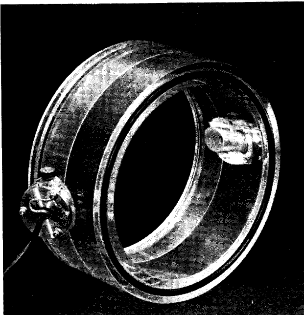
Figure 7. Segment of perspex pipe with the acoustic transmitter and receiver.
